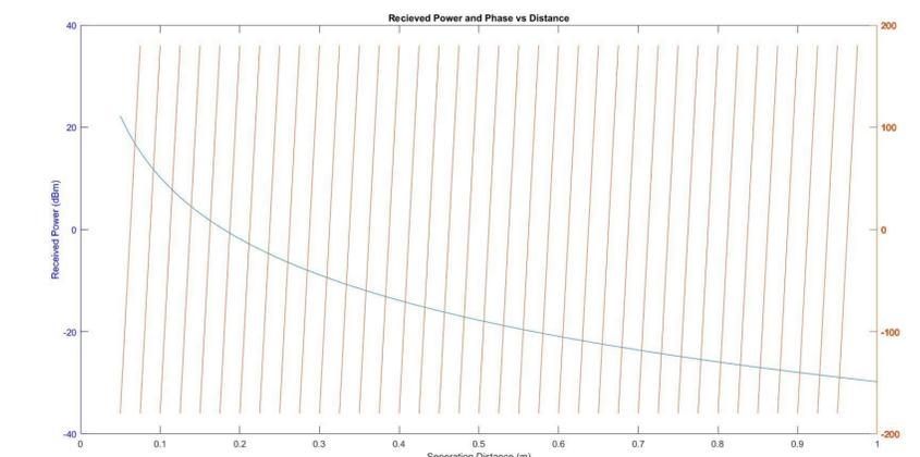
Figure 5: Received backscatter phase and magnitude. 1 watt radiated power starting at 5 cm separation distance.
