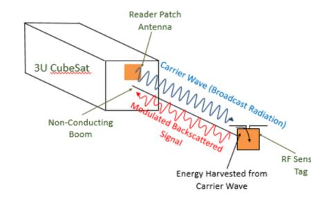
Figure 4: RF Backscatter Communication
