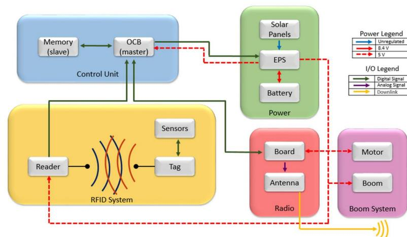
Figure 2: RFTSAT Systems Summarized in a Functional Block Diagram
